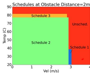
Fig. 2: The set of schedules generated. CAuWS can precompute multiple schedules for varying physical parameters, handling changing conditions. Schedule 1 is fast but uses more energy scheduling all 3 tasks on all 3 devices simultaneously, while Schedule 3 is the reverse, only using the CPU and DLA.
